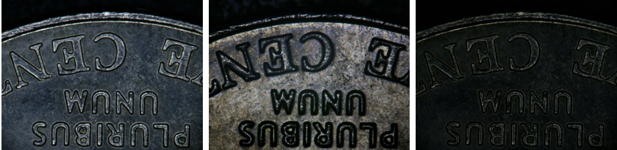
Figure 17 From left to right, there are three pictures of coins taken under left) LED Direct Ring Light illumination; middle) LED Direct Ring Polarization Light illumination; right) Coaxial Light illumination
