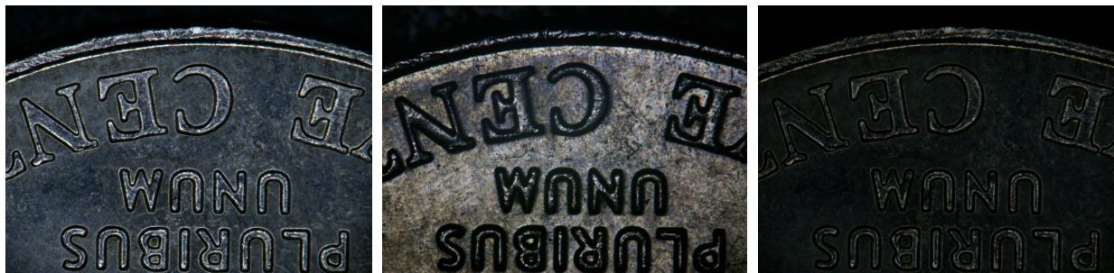
Figure 9 From left to right, there are three pictures of coins taken under left) LED Direct Ring Light illumination; middle) LED Direct Ring Polarization Light illumination; right) Coaxial Light illumination
