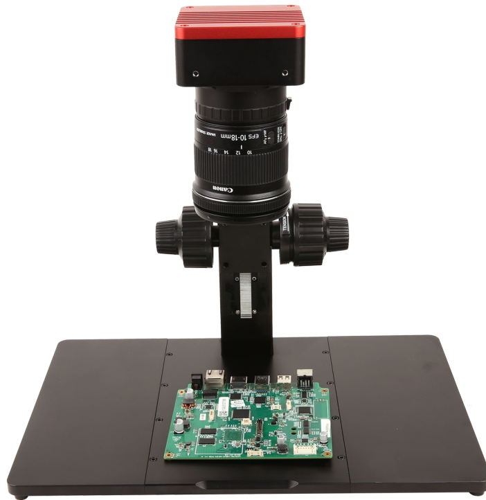
Figure 1-4 IUCXXX-AFU-EF camera, Canon EF lenses with TPS-600 fine focus bracket
