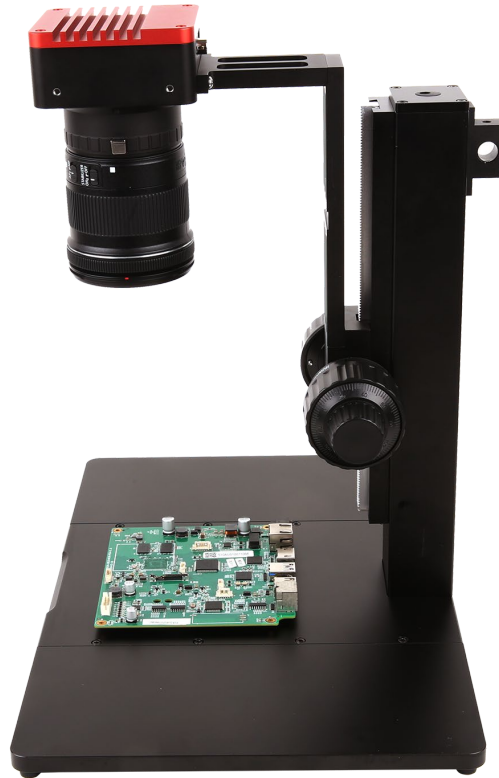
Figure 1-6 IUCXXX-AFU-EF camera, Canon EF lenses with TPS-600 fine focus bracket
