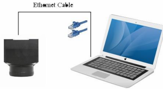
Figure 15 Connecting the X7FCAM4K16MPA_EFL Camera with Ethernet Cable to the PC
