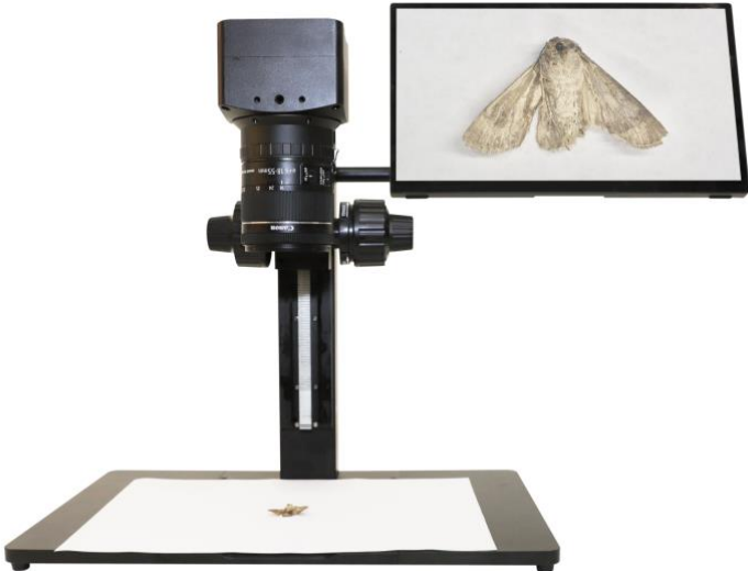
Figure 5 TPS-600 Bracket+X7FCAM4K16MPA_EFL+Canon EF-S 18-55mm f/4-5.6 IS STM+HDMI 4K Monitor
