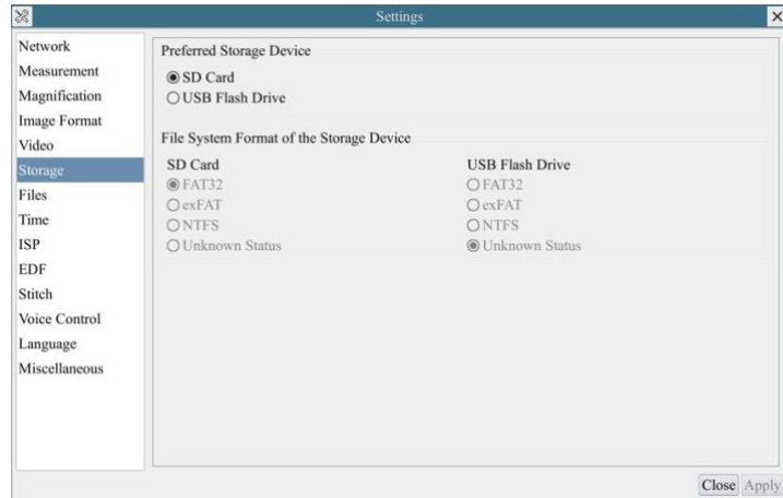
Figure 31 Comprehensive Setting of Storage Page
