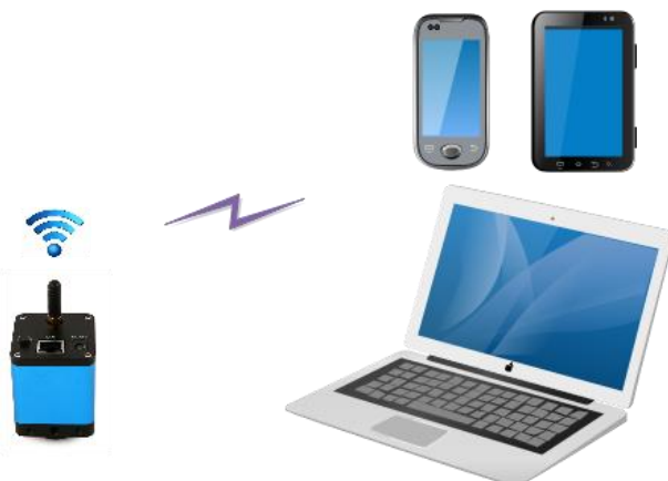
Figure 4 The PC or Mobile Device Connect to the Camera through WiFi AP Mode
