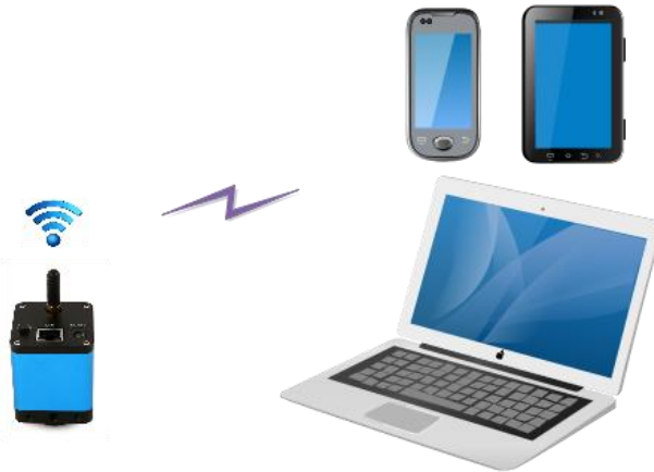
Figure 2 The PC or Mobile Device Connect to the Camera through WLAN AP Mode
