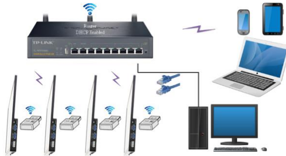
Figure 10 Multi AIOCAM4K Series All-in-One Cameras Connecting to the Router through the WiFi Style
