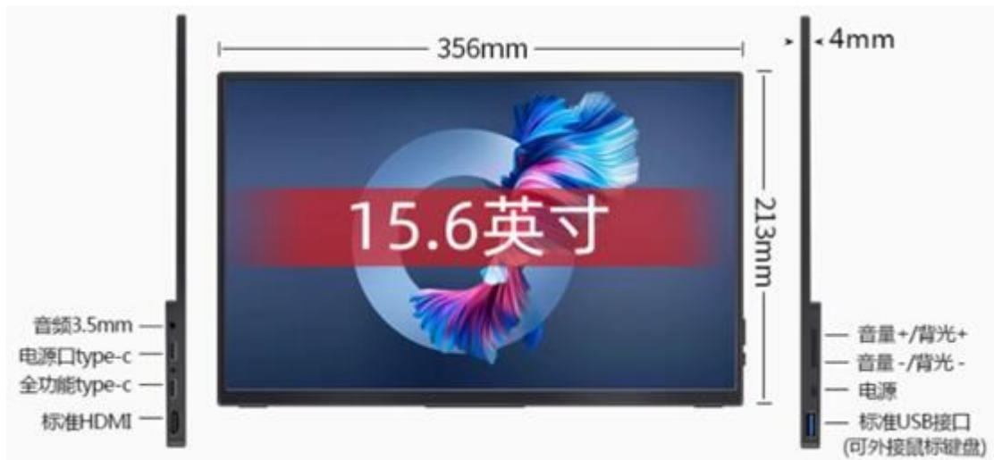
Figure 3-14 Dimension, Interface and Control Button of TPHD1080P156A Displayer
