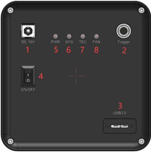
Figure 12- 6 MAX251& MAX151&MAX102 Camera interface diagram
