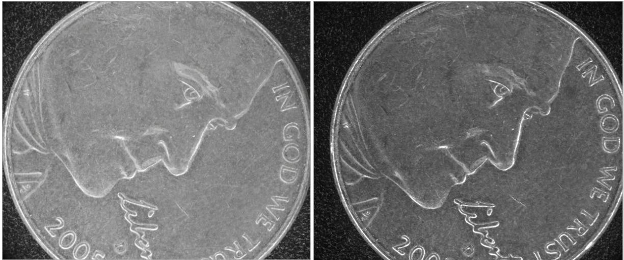
Figure 5- 70 Ordinary camera (left) compared with polarizing camera (right) metal surface effect
