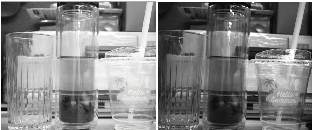
Figure 5- 68 Comparison of plastic surface effects between ordinary camera (left) and polarizing camera (right)
