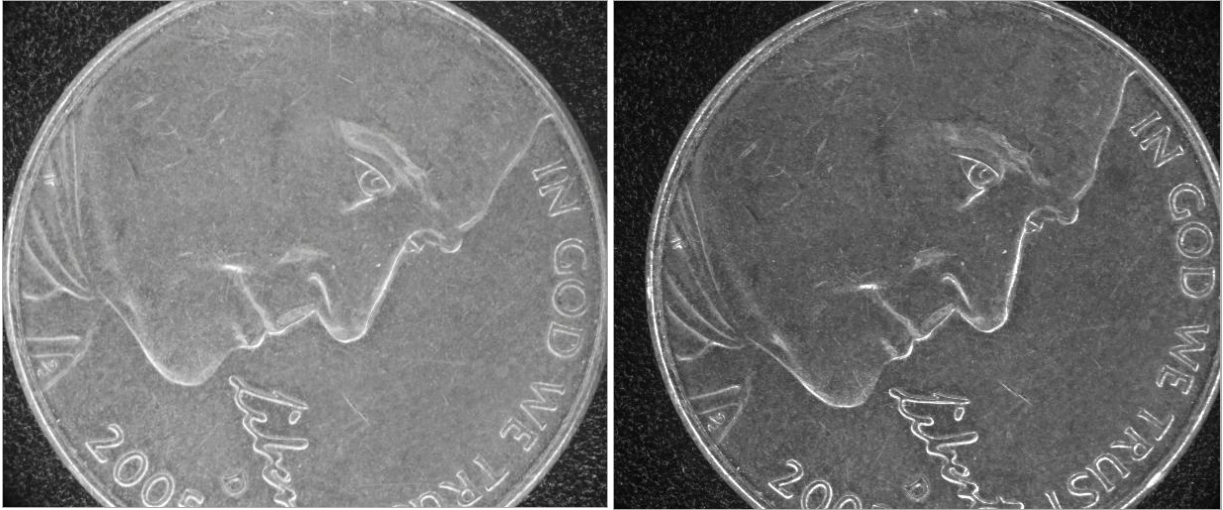
Figure 5-92 Ordinary camera (left) compared with polarizing camera (right) metal surface effect
