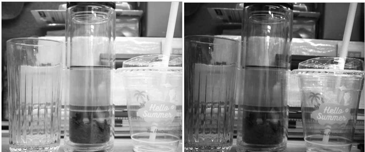
Figure 5- 90 Comparison of plastic surface effects between ordinary camera (left) and polarizing camera (right)
