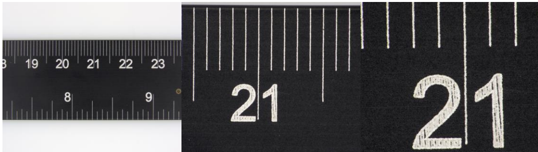
Figure 4 Images of ruler taken with TZM015120-W4100-TV4100 under LED Direct Ring Light illumination left) 0.15X, middle) 0.6X, right) 1.2X
